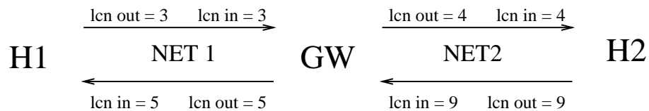
Figure 4.11: Data transfer through a gateway
