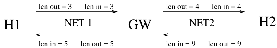
Figure 4.11: Data transfer through a gateway
